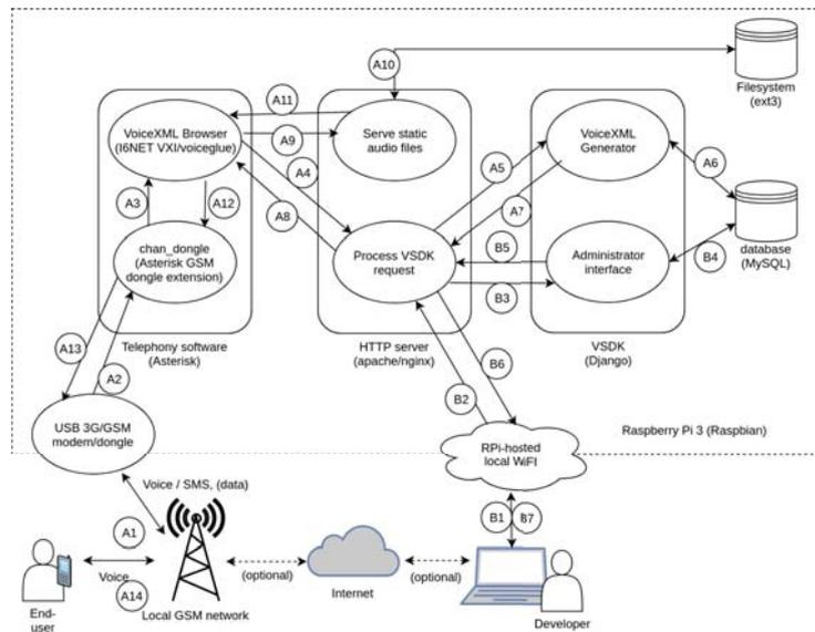
Figure 1: Overview of the Kasadaka system architecture
