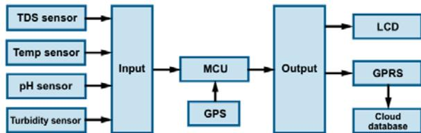
Figure 1: Block diagram of first iteration device
